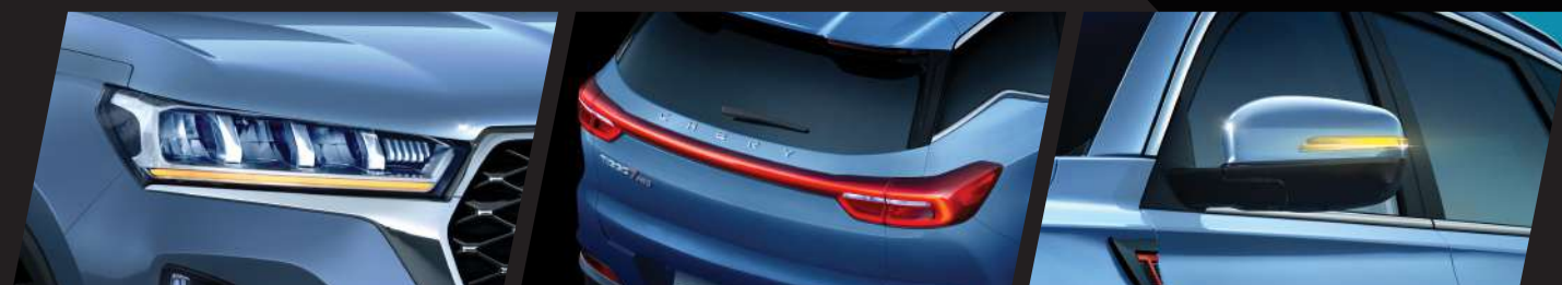
Daytime Running Lamps and LED Headlamp with Electric Height Adjustment
